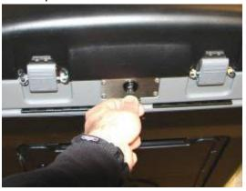
• Using the barrel key unlock the lock on the front of the scanner.
