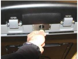
• Using the barrel key unlock the lock on the front of the scanner.
