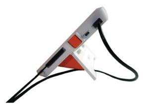
• Inside the bottom of the DS200 scanner is a square black and orange soft case containing the ExpressVote printer. Open the case and remove the printer and the two black cords.
