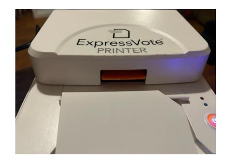
When printing is complete, pull the activation card from the printer.
